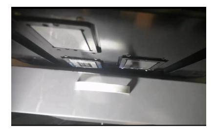
7. Adjust the Print Table height and then Print Test from software to check the nozzle status good or not. If good, you can start to print job, if not good, repeat step 5 and 6 .
