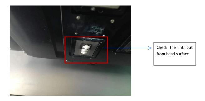
6. Wipe the head surface slightly with cleaner cloth after press cleaning
