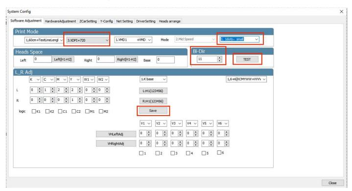
Calibration: click test, print the test strip, make sure the color blocks at position 0 overlap, find the value of the overlapping color block, and then  $\pm$  value base on the original value, for example, if the alignment value is  $\pm 2$ , and original value is  $\pm 11$ , So  $\pm 11$ , put  $\pm 13$  and save
