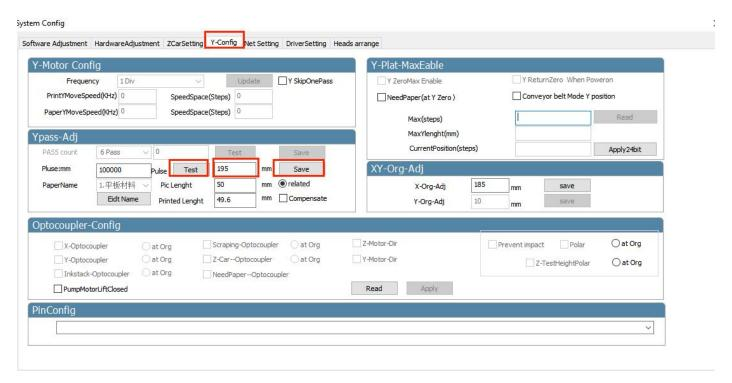
Click "Test" to print the test strip, measure the distance between the color patches as below, fill in the value, and save (\*only click one time save)
